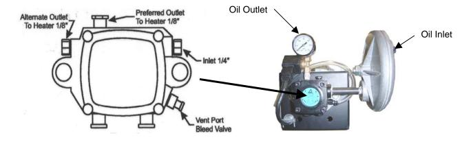
Figure 4 – Oil Pump Diagram
